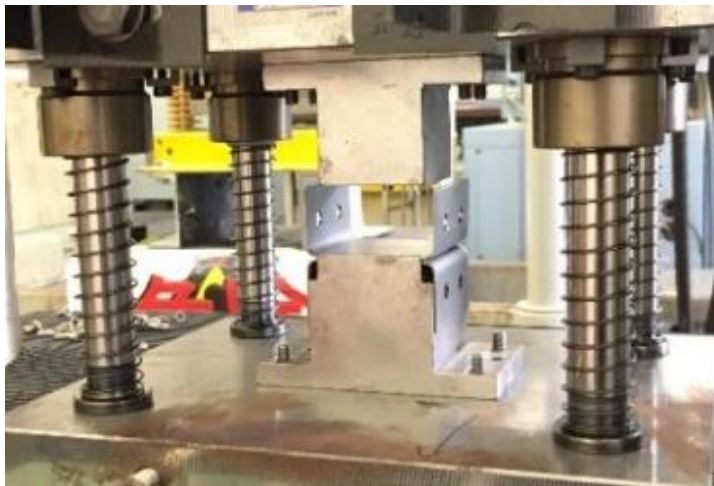
(c) Specimen attached to 30t universal testing machine
